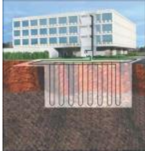
Figure 2: Vertical Loop System
